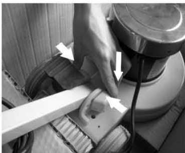
Step 7 - Put screw box into chassis.
